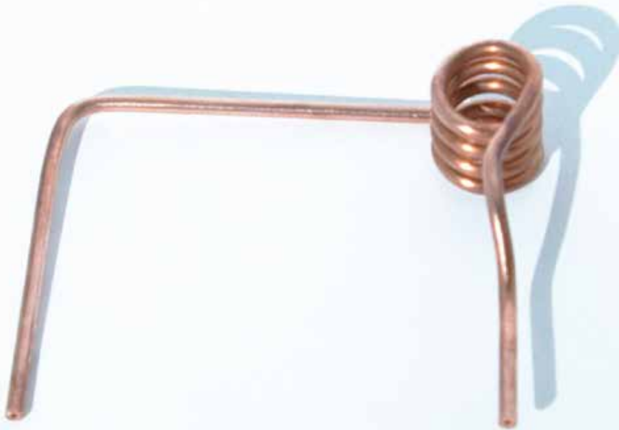
Simple inductor for heating small split mold cavities. Through oriented temperature management and influencing the induced eddy currents, inductor design can be simplified (© IKFF)
