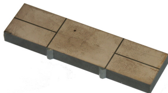
Fig. 10: Dual mode resonator [3]
