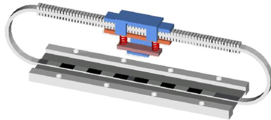
Fig. 2: Linear travelling wave motor with ring-type stator
