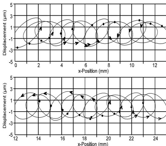
Fig. 7: Trajectories of points located on top of the teeth ( $f = 51001,3$  Hz)
