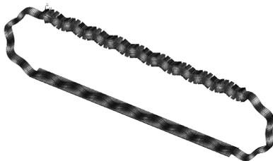
Fig. 3: Bending mode shape of ring-type stator
