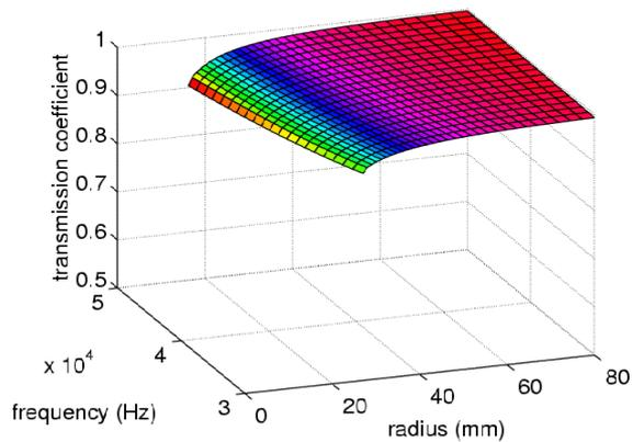
Fig. 5: Transmission of bending travelling wave into curved portions (magnitudes only)
