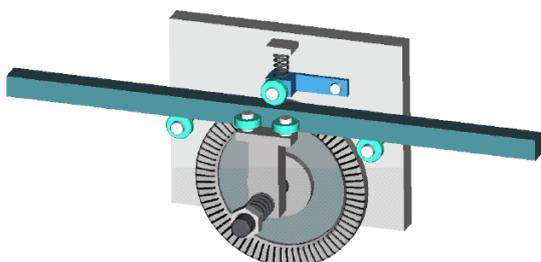
Fig. 1: Linear travelling wave drive with a straight rod pressed tangentially onto rotational symmetric stator
