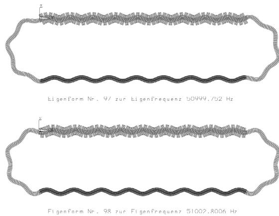
Fig. 4: Pair of orthogonal bending mode shapes
