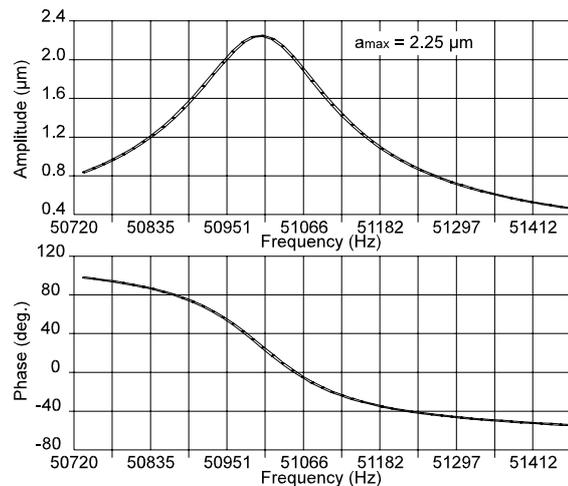
Fig. 8: Resonance curve of the travelling wave (electrically excited by 80 V)
