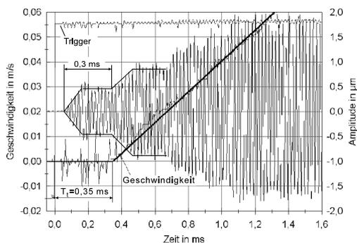
Fig. 11: Correlation between the stator's oscillations and the slider's acceleration
