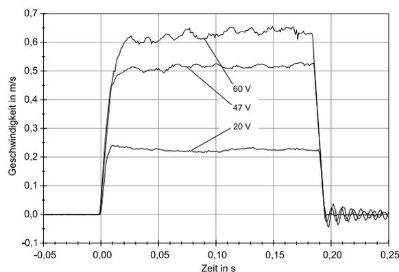
Fig. 9: Velocity versus time, depending on the exciting voltage output
