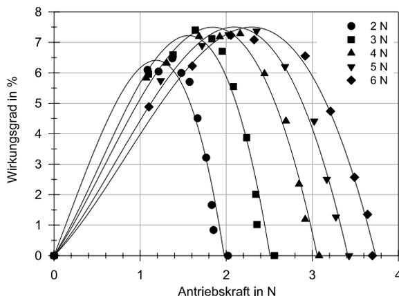
Fig. 12: Efficiency versus propelling force, depending on the compressive force between the slider and the stator
