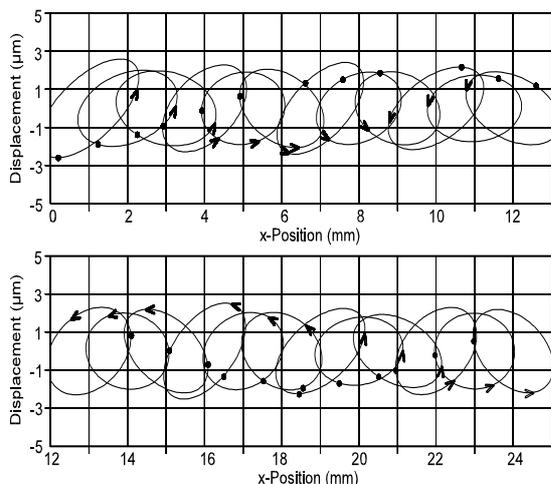
Fig. 6: Simulated trajectories of points located on top of the teeth ( $f = 51001,3$  Hz)
