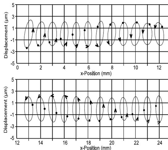
Fig. 4: Simulated trajectories of points located on bottom of grooves ( $f = 51001,3$  Hz)
