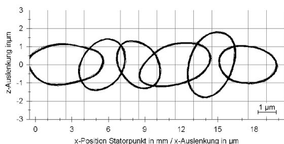
Fig. 7: Measured trajectories at a height in the middle between the grooves and the surface ( $f = 48100$  Hz)
