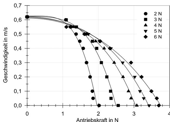
Fig. 8: Characteristic curves of velocity versus propelling force, depending on the compressive force between slider and stator ring
