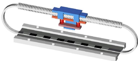
Fig. 1: Linear travelling wave motor with ring-type stator
