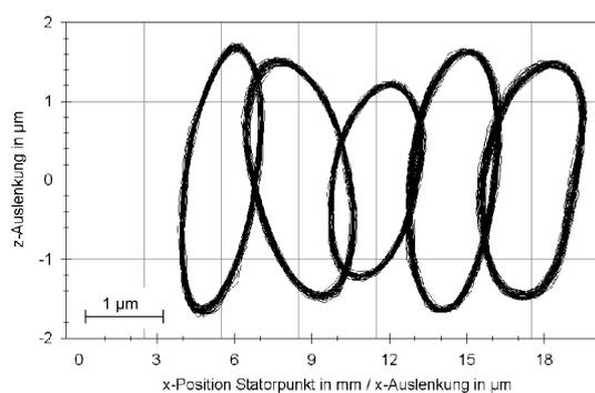
Fig. 5: Measured trajectories of points located on bottom of grooves ( $f = 48100$  Hz)
