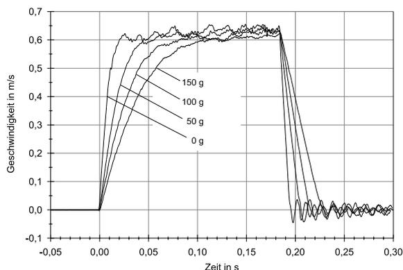
Fig. 10: Velocity versus time, depending on the mass load attached to the slider
